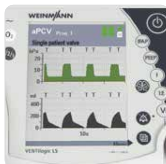
Pressure and volume curves with auto-scaling function
