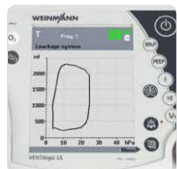
Pressure/volume Loop with auto-scaling axes
